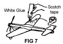
If the foam cracks, apply small amount of white glue to the break and hold firm with scotch tape or pin until dry. Remove the tape or pin when you are ready to fly again (FIG 7).
